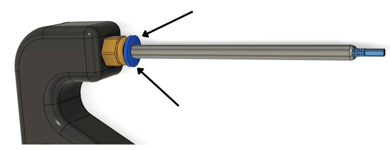
To install, gently slide the feeler into the hole past the locking mechanism. Then firmly press the feeler into its bore.
